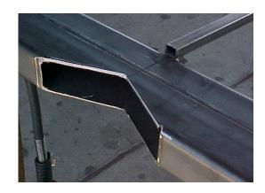
Step 1: Cut a "V" notch in your bottom rail using a grinder and 4 1/2" x .040 x 7/8" cutting wheel (or alternative method)
