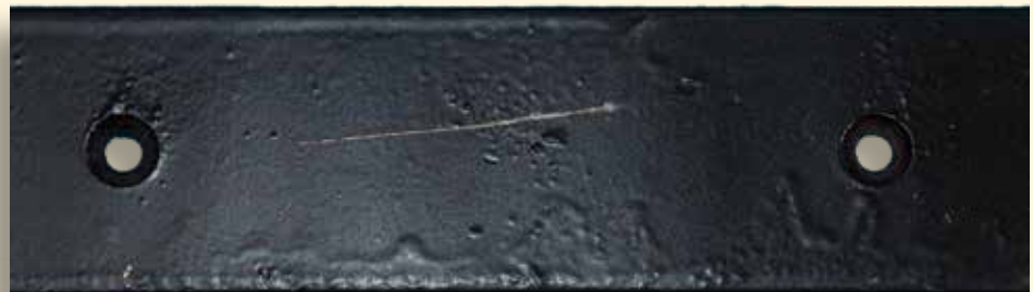
Close up of Deliberate Scratch shows little rust, no rust migration, and no detachment of the surface coating
