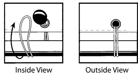
4. Place straps through grommets and around sidewall pipe as seen above (Figure 2). Sidewall pipe should then be pulled down until the cover is pulled tight. Then the clamps may be tightened.
