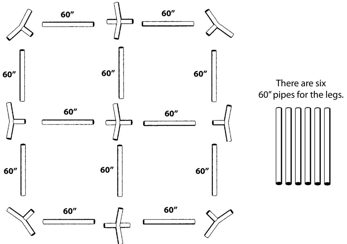
2. Start with the center and complete the center frame first. Then assemble each side.
