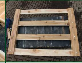
Measure distance between stiles and cut upper rail to f t. Place in position but do not fasten at this stage.
